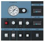
Inlet temperature, outlet temperature are displayed digitally. Condition setting dials and stage level control switch are located on the front panel for easy use.
